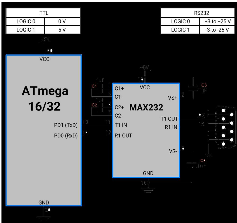
ATmega16/32 Serial Interface Connection Diagram
